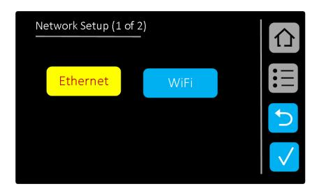
In the above screen select **Ethernet**. The selected network connection is highlighted in yellow. Press the **Accept** button to confirm your selection and move on to the next screen as below.
