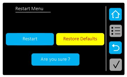
Press **Are you sure ?** to enable the **Accept** button. Now press **Accept** to complete the restore defaults process and reboot the unit. This will reset all network settings and other stored parameters to the values as in section 2.6.
