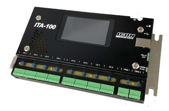
The basic operation is that analog signals are digitised by the on-board analog-to-digital converter (ADC) and stored in internal memory. This data can be passed over a 100base-T ethernet cable or a WiFi 802.11b/g/n network to a host computer for processing and display.
