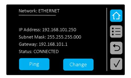
Pressing **Ping** enables you to ping other devices on the network. This is useful, for example, in ensuring that a host computer is reachable. A screen similar to the one below appears.
