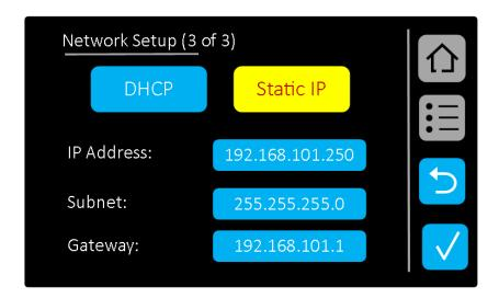
This screen shows that **Static IP** has been selected. Pressing on any of the buttons below brings up the keyboard screen and you can adjust the settings as required. Press **Accept** to confirm.
