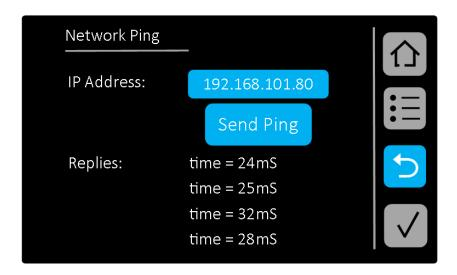
Pressing **Send Ping** sends a ping to the IP address specified on the screen. Replies or other unreachable messages will appear. An example of a successful ping is shown above. If you wish to change the address being pinged, press on the IP address (in this example **192.168.101.80**) and the keyboard screen will appear enabling you to change the IP address.
