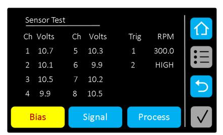
The first screen shows the bias voltage levels of all the dynamic channels together with status of the trigger inputs. If an accelerometer is not connected or the cabling
