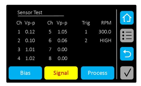
The voltages shown are the peak-to-peak voltages measured on the corresponding channel. Knowing the sensitivity, for example, of the accelerometer connected, the value in g's can be calculated. The RPM readouts are as in the BIAS screen. The measurements continually refresh.
