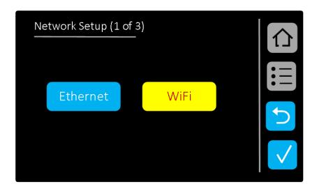
In the above screen select **WiFi**. The selected network connection is highlighted in yellow. Press the **Accept** button to confirm your selection and move on to the next screen as below.
