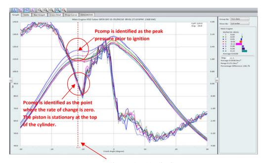
The cursor is positioned at the desired TDC point. In this case it is 11.5 degrees from the correct angle.
