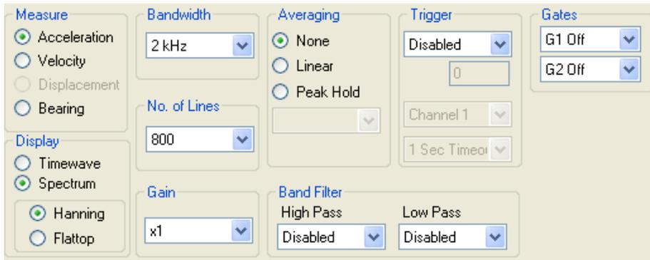
**Measure:** The type of measurement is defined here. The options are context sensitive depending on the type of sensor selected. For example, you cannot measure acceleration when using a proximity probe. The table below shows the types of measurement that can be taken with each type of sensor.
