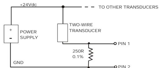
A load resistor is connected between pins 1 and 2 of the ITA-1. This resistor can be mounted on the connector itself or on a terminal strip mounted in the enclosure. A value of 250R is selected as this will give a 5V output at full scale range of 20mA. Alternatively, a 100R resistor can be used which will give a maximum output of 2V. Setting the gain of the ITA-1 channel to 5 will give a 10V range internally to the ITA-1. Note that the input range with a 250R
