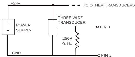
The diagram above shows a typical 3-wire transducer arrangement. Again, the power supply can power multiple transducers but a higher rated supply current may be required due to the quiescent current of the transducers.
