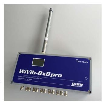
The *WiVib's* incorporate an ICP power supply on each of the dynamic channels so that any standard compatible accelerometer can be connected. Alternatively, the inputs can be AC coupled to interface with buffered signals from other systems. High-resolution acceleration and velocity measurements can be made, together with bearing condition using the built-in demodulator or "enveloper" as it is sometimes called. Accelerometer bias voltage checking is incorporated.
