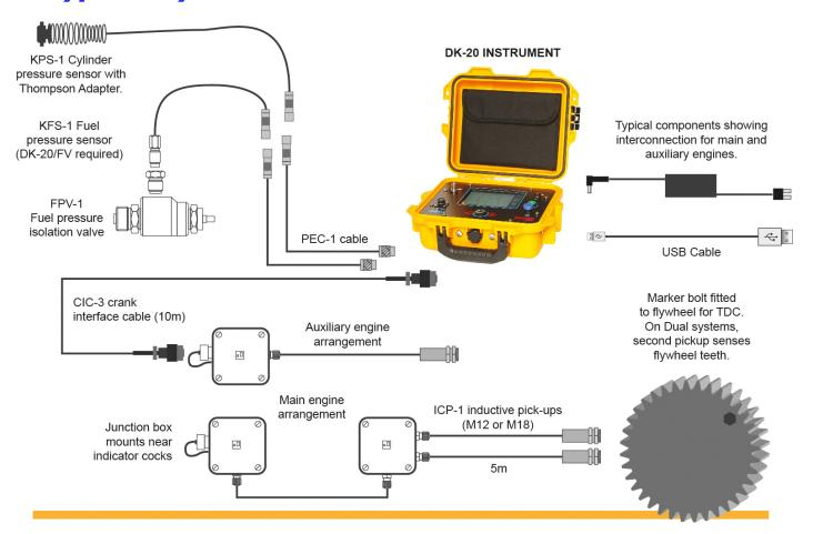
The *Doctor* instrument is available in two versions, namely the single-channel DK-20 for cylinder pressure only measurements, and the two-channel DK-20/FV which incorporates a second channel for simultaneous fuel or vibration measurement. Fuel injection sensing can detect issues with injectors while vibration sensing with an accelerometer can detect valve timing within the cylinder. The diagram above shows how the sensors connect to the DK instrument.
